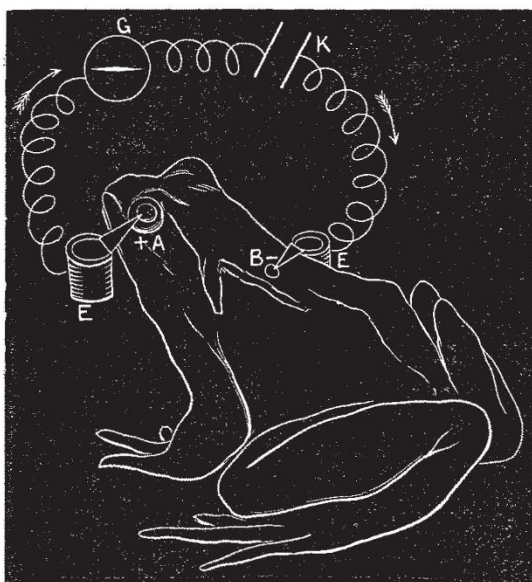
Diagram showing arrangement of apparatus in the experiment on eye of frog. A, Eye showing the electrode, E, in contact with it. B, Skin removed, and subcutaneous tissue in contact with other electrode, E. K, Key. G, Galvanometer. Arrows indicate direction of current. Cornea, positive. Back, negative.
