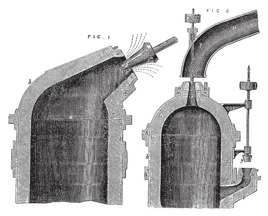
mouth of which the iron hoop, c, is riveted; while d is a flanged iron ring bevelled on the inside, and secured by screwed studs or cotter bolts to the hoop, c. A moulded ring, e, of firebrick or other suitable refractory material, forms the escape opening or mouth of the vessel; it is retained in place by means of the flanged ring d
