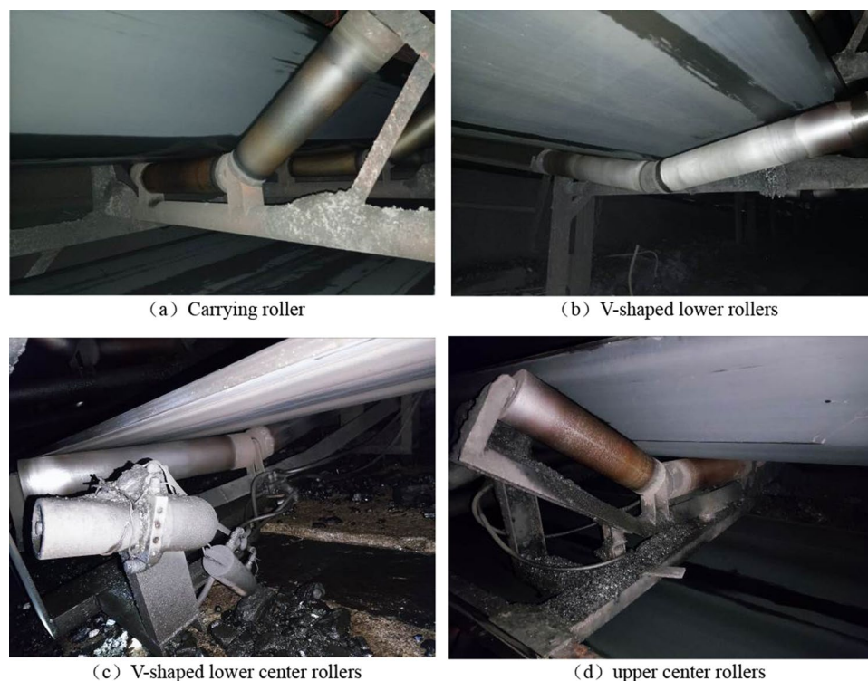
Figure 6. Roller type. (a) Carrying roller, (b) V-shaped lower rollers, (c) V-shaped lower center rollers, (d) upper center rollers.
