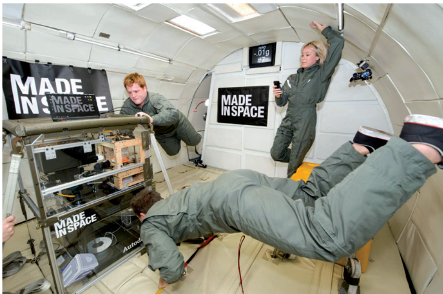
Engineers test a 3D printer under microgravity conditions aboard a modified aircraft in parabolic flight.
