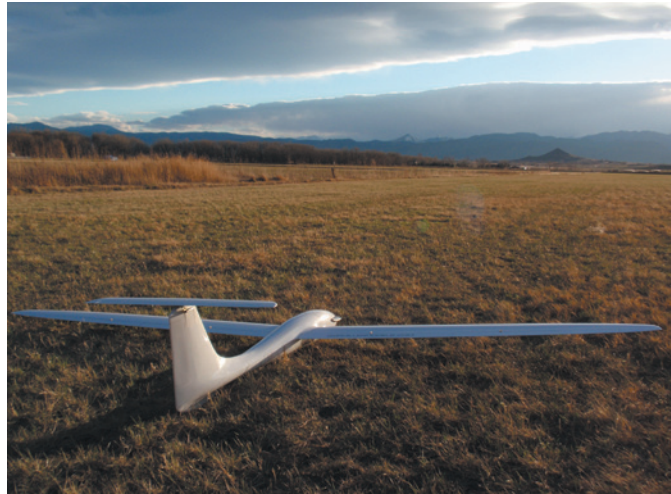
The Tempest in Colorado was designed to collect data from severe storms.
