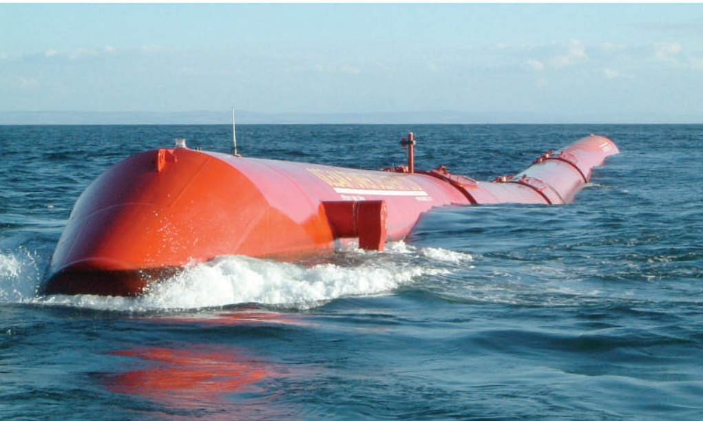
Sea snake: Pelamis has been testing its 750-kilowatt wave machine in the Orkney Islands in Scotland.
