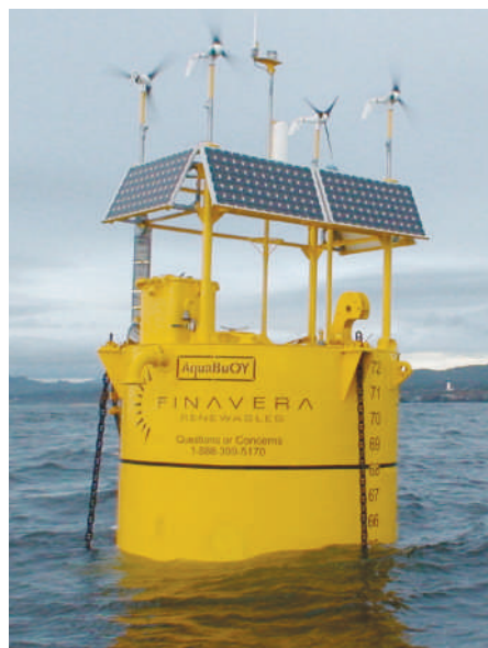
Bobbing buoys: Finavera's Aqua Buoy used to harvest energy from the waves near Oregon.
