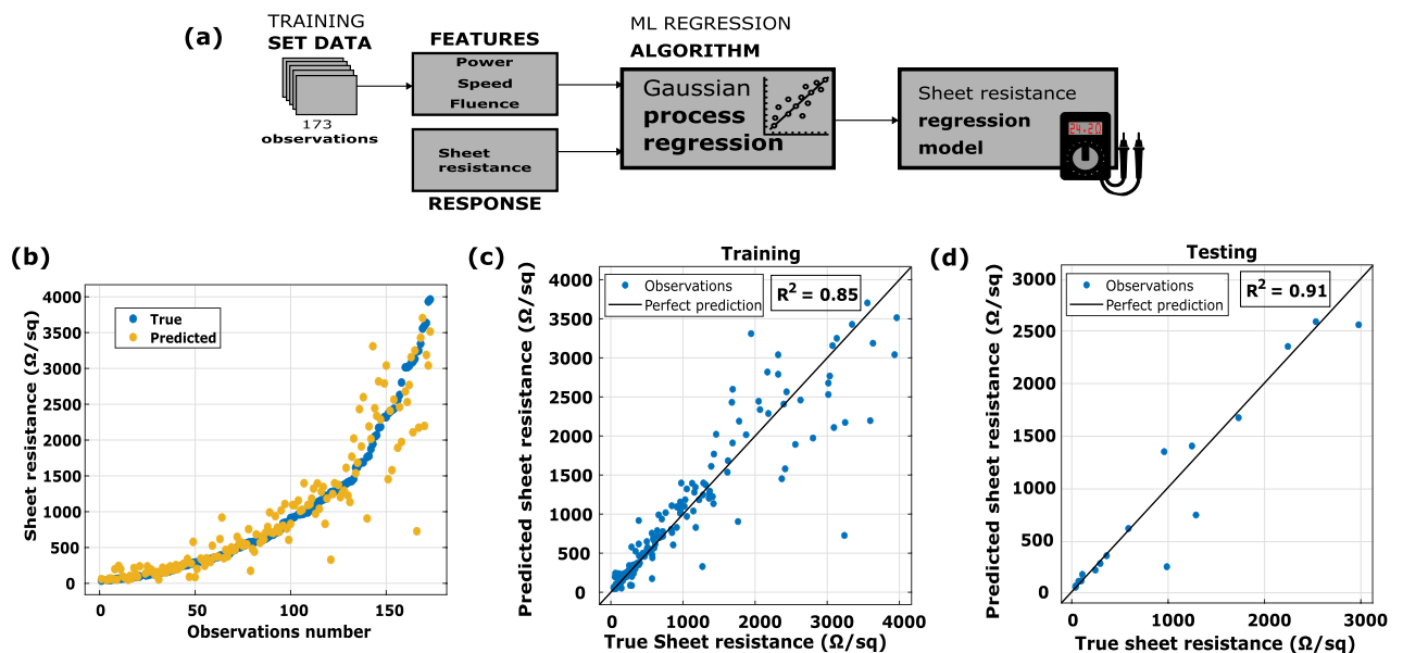
Figure 6. Schematic illustration shows (a) a block diagram of the estimation sheet resistance of LIG, (b) scatter plot and correlation plots of the (c) training and (d) testing procedures.
