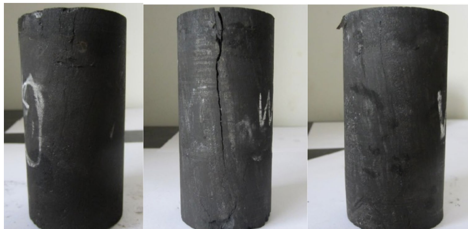
Figure 15. Failure modes of coal samples G1, W1 and W3.
