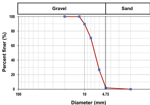
**Figure 4.** Particle size distribution of steel slag.
