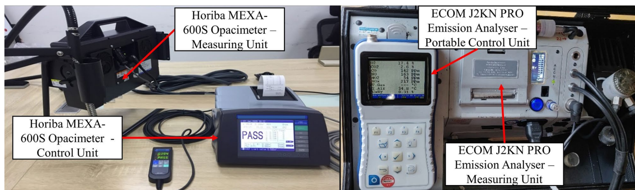
Figure 4. Exhaust gas analysis measuring equipment.
