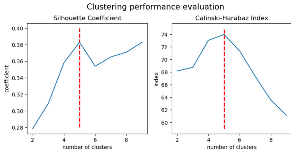
Figure 4. Clustering performance evaluation. To determine the optimal number of clusters in the hierarchical cluster analysis a consensus of two different methods were used. The mean Silhouette Coefficient (on the left) is calculated over mean intra-cluster distance divided by the minimal inter-cluster distance to the nearest cluster. Positive values indicate a dense clustering whereas negative an incorrect clustering. The Calinski–Harabaz index (on the right) is the ratio of the sum of distances squared between and within the clusters. A high index indicated a dense and well separated cluster. Both methods indicate an optimal number of clusters of 5.
