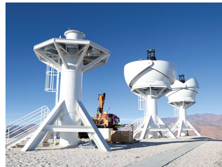
Fig. 1 | The first two BlackGEM telescopes installed in their clam-shell enclosures at the European Southern Observatory's La Silla Observatory in August 2019. The third tower is awaiting the third dome, which was shipped to Chile in November 2019.
