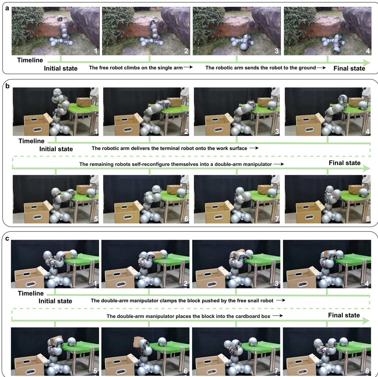
Fig. 9 | Snail robot swarms form different kinds of robotic arms to perform manipulation tasks. a Flow diagram of an outdoor single-arm experiment. b A single-arm manipulator made of snail robots can reconfigure itself into a dual-arm
