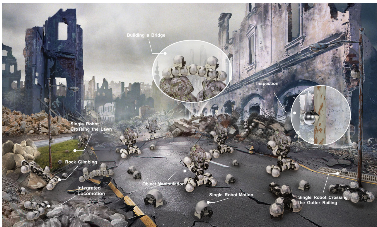
Fig. 1 | Overview of the snail robot swarm system. A depiction of the mission profile: A single snail robot can traverse most outdoor terrains and even climb metal poles to carry out monitoring tasks. When working together, multiple robots
