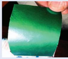
change the pitch of the photosensitive cholesteric mixture, and thus tune the spectral response of the mirror's reflection across the visible range — longer durations of ultraviolet exposure give shifts to longer wavelengths. Furthermore, by using a mask during ultraviolet exposure, an array of miniature reflectors with different spectral properties can be realized; for example, a pattern of red, green and blue mirrored pixels can be realized on the one substrate.
