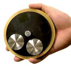
compact, light-weight generator (pictured), consisting of a copperplated disk that spins and rubs against a static base containing a layer of electrodes and a conducting surface. The device can harvest mechanical energy from gentle wind, tap-water flow and normal body movements.
