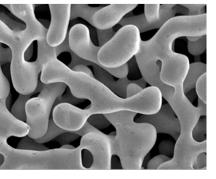
unknown, the authors think that the adsorbed anions may be slowing down the movement of inherent defects at the surface of the nanoporous gold, enhancing the material's strength. They anticipate the development of a material that can be made ductile during moulding or fabrication, and tuned to the strong state when desired.
