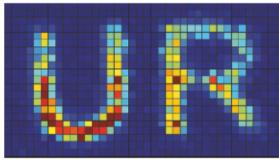
'UR' pictured above — recorded in light pulses can indeed be 'stored' after a fashion. Light passing through caesium gas is slowed down massively, delaying a pulse by up to 10 nanoseconds and thus allowing it to be 'held onto' for longer than normal. MERICANPHYSICALSOCIETY
