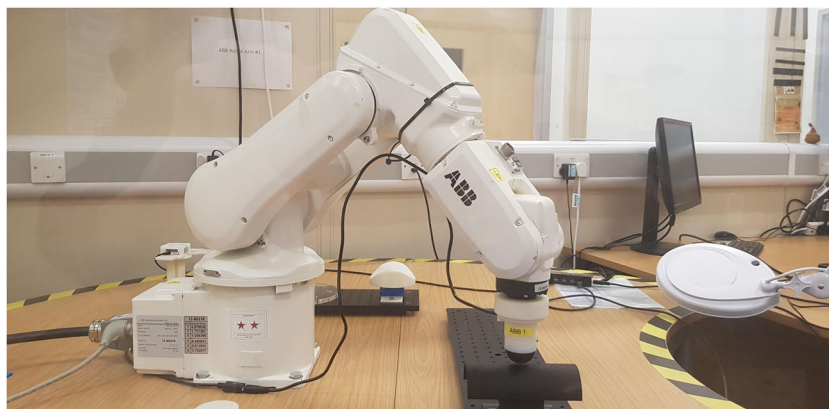
Fig. 3 A robot arm equipped with a TacTip sensor. TacTip (black semi-sphere) is developed to create a sense of touch for the robots so when the robot touches a surface of an object it can detect patterns and shapes based on deformation of the TacTip sensor. (Credit: Mehdi Sobhani).
