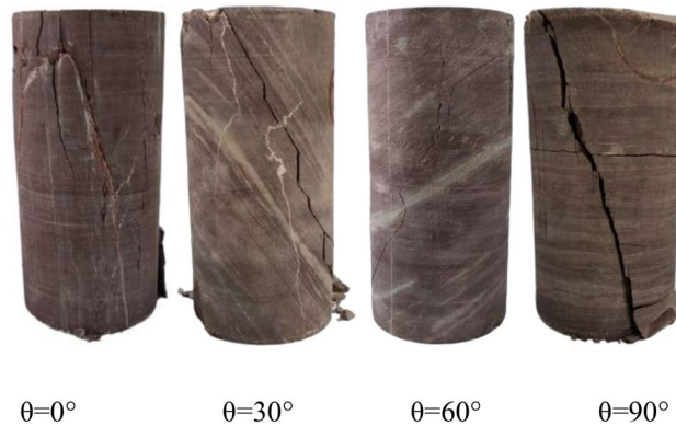
Figure 2. Diagram of crack propagation of specimen.
