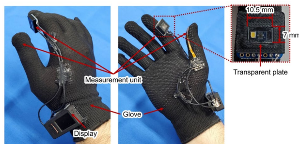
Figure 2. Prototype wearable CRT measurement device: Medic Hand.
