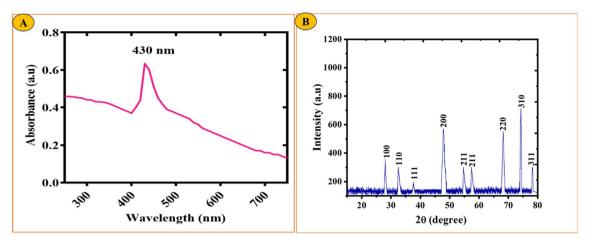
**Figure 2.** (A) The UV visible spectrum of biologically synthesized AgONPs (B) XRD spectra of *R. capitata*-mediated AgONPs.
