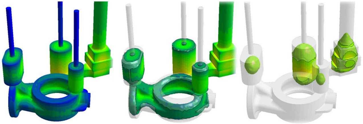
Figure 15. Solidification simulation of the new reinforced sample (own design for the process).
