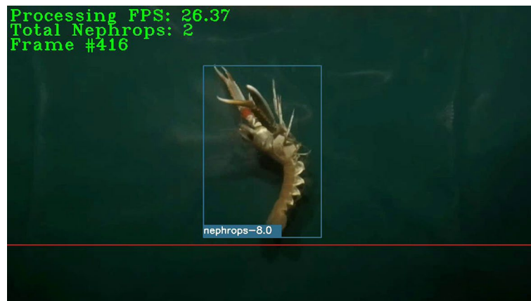
Figure 1. A sample processed frame showing the horizontal level (red line), bounding box and some information about the status of the processing.
