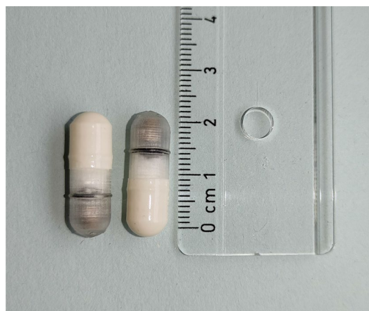
Figure 5. Capsule for Sampling (CapSa) device a rule is included for size comparison.
