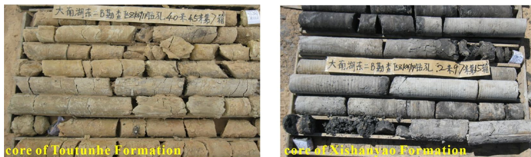
Figure 6. Cores of Toutunhe Formation and Xishanyao Formation (cores from ZK4911 borehole) (This image is taken by Jingzhong Zhu and Dongding Li during field sampling at Dananhu No.7 coal mine).
