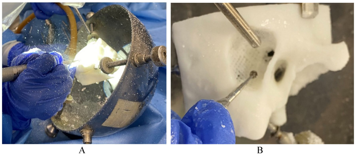
Figure 7. Simulation of the mastoidectomy simulator considering mechanical properties. (A) The mastoidectomy simulator was drilled while fixed on a jig. (B) Front view of the mastoidectomy simulator with the air cell removed.
