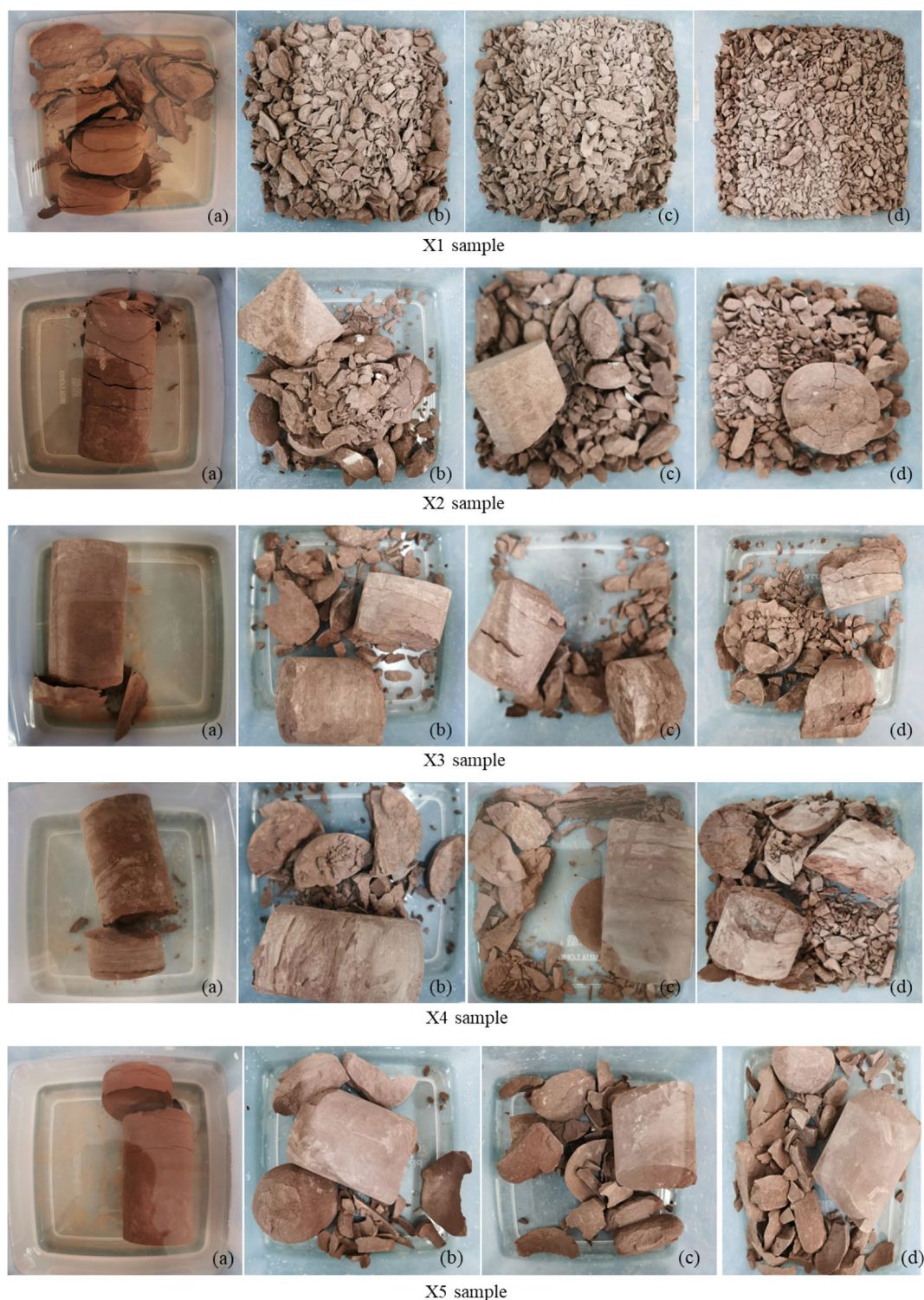
Figure 5. Disintegration of X1 sample: (a) cycle one; (b) cycle three; (c) cycle five; and (d) cycle ten.
