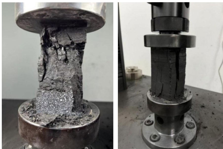
Figure 7. Experiments on the uniaxial compression process of a coal body.
