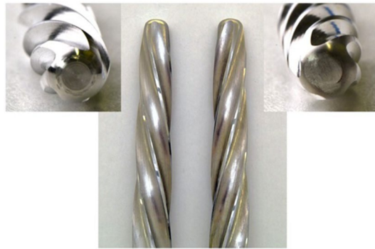
Figure 2. Overview and microscope photo of the left- and right-cutting conical reamer from LINK with a diameter of 17 mm.
