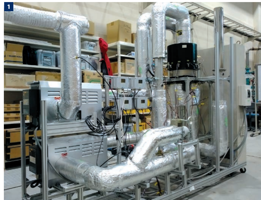
▲ 1. Direct air capture technology from Kanazawa University sucks up ambient CO 2 from the atmosphere.
