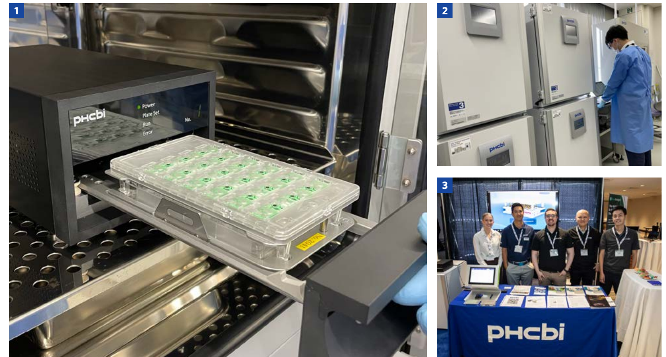
▲ 1. A LiCellMo sensor module attached to a common commercial plate is placed in the Detector pre-installed within the CO 2 incubator. 2. A researcher is checking the real-time measurements using the touch-panel controller. 3. PHCbi team at a sponsored conference by Stem Cell Network in Vancouver, BC, Canada to discuss the developing new technology, LiCellMo, a live cell metabolic analyzer.
